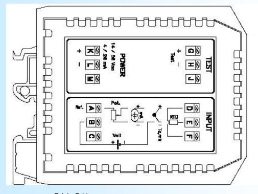
D (+), E (-) B (+), E (-) mV input: V input: D (+), E (-), internal 2 ohms shunt mA input: D and F(+), E (-) Resistance 2 wires input: D (+), F (line), E (-) D and F(+), E (-) Resistance 3 wires input: PT100 2 wires input: PT100 3 wires input: D (+), F (line), E (-) Tc input: D (+), E (-) A (+Réf), D (+), E (-) Potentiometer input: K (+), L (-) G (+), H (-) Power supply / analog output: Test pins:
